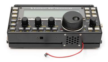
9. Combine PART2 and the KX3 transceiver together with 2 screws (4-40\*1/2, American Standard).
