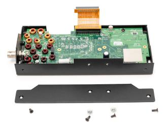
6. Take out PART1 aluminum alloy accessories and install the parts with reference to the picture below.
