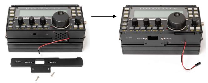
10. Combine the PART3 and the PART2 together with 2 screws (M3\*5mm).
