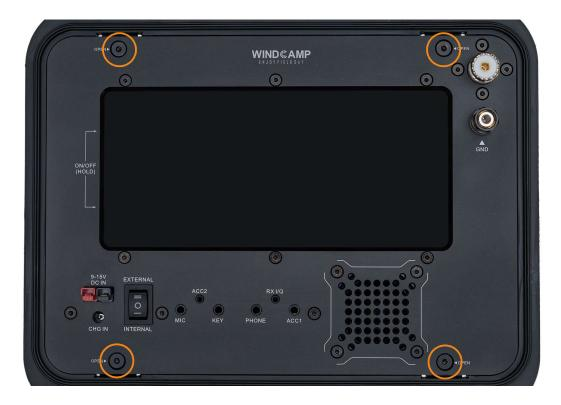
2. Use the M2 hex key to loose the six screws inside the yellow circle and then the internal aluminum alloy parts of PART1, PART2, PART3 and PART4 could be removed. After removing the fittings and screws, place them properly for later use.
