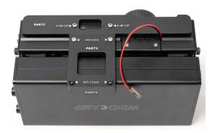
12. Combine the KX3 transceiver and the Safety Box panel together with 6 screws (M3\*8mm, black).
