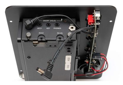
14. There are 5 jacks(2.5mm/3.5mm) on the circuit board and they are labeled as MIC,KEY,ACC1,ACC2 and RX I/Q respectively. Please choose the related cable and connect them to the KX3 transceiver correspondingly.
