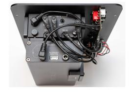
17. Connect the antenna port of KX3 transceiver to the antenna port of the Safety Box panel with the provided RF Connector Cable.
