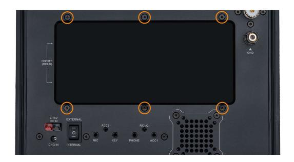
3. Remove the thumb screws from the left and right side-plate of the KX3 transceiver, as well as the foot frame.
