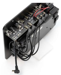
15. Connect the KX3 transceiver antenna port to the antenna port of the Safety Box panel with the provided RF Connector Cable.
