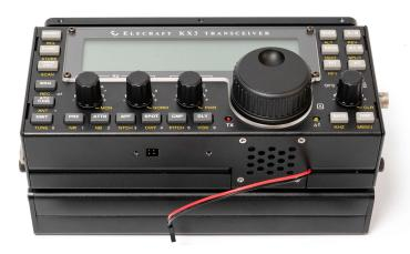
9. Combine PART2 and the KX3 transceiver together with 2 screws (4-40\*1/2, American Standard).
